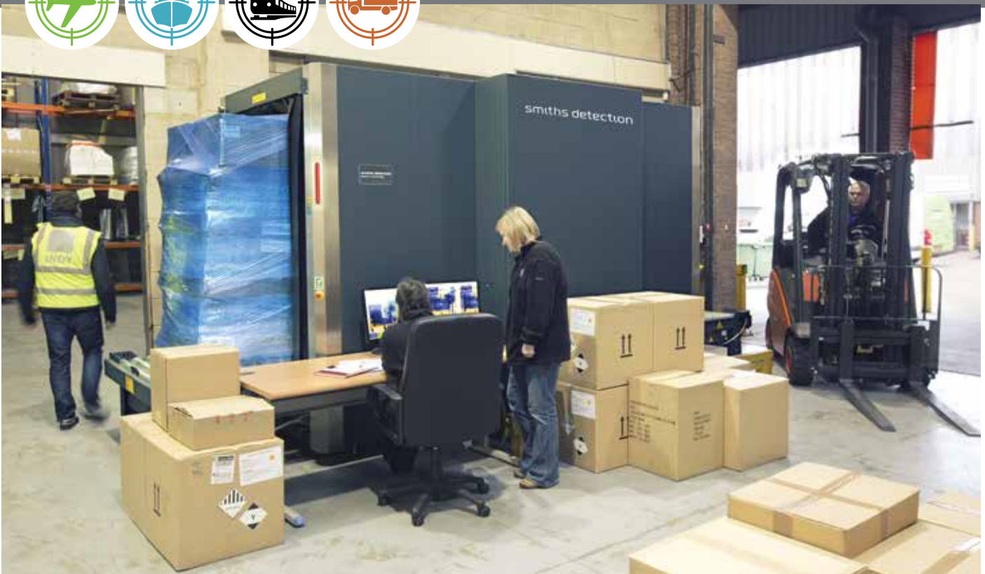
Smiths Detection's HI-SCAN 145180-2is, shown above, has two 160kV generators in 90° opposition providing a horizontal and vertical view of the object for shortened inspection time and high-quality images, the company says. Smiths Detection image.
