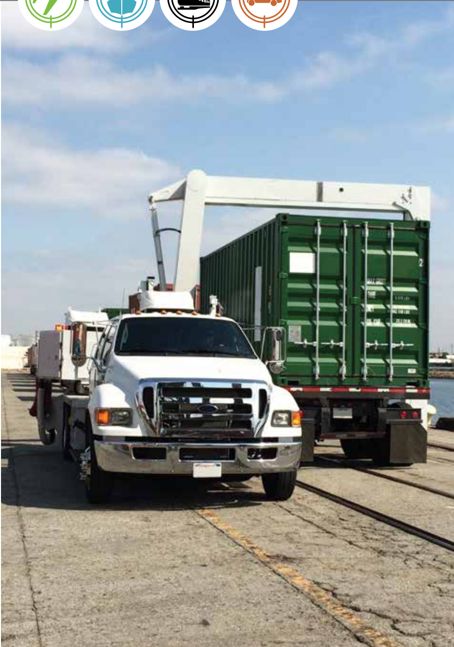
The Leidos VACIS MLX Mobile Light X-ray Inspection System features a short wheelbase and light weight for better maneuverability and handling, an industrial chassis designed for firetruck duty, a global support network and an advanced high-energy imaging system with material discrimination, the company says. Leidos image.
