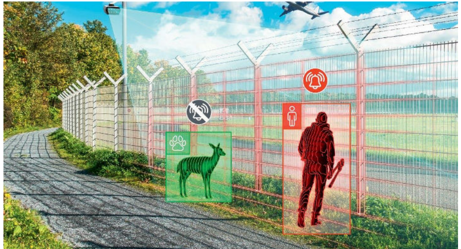
AI-based camera technology can automatically classify objects at the perimeter and is used by airport managers for visual verification. Dallmeier image.
