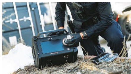
Teledyne FLIR Defense says its Griffin G510x portable chemical detector is specifically designed to analyze and identify explosives and narcotics (such as fentanyl and its analogs) within five minutes. Teledyne FLIR Defense image.
